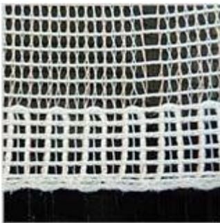
Knitted fabric with meander-shaped, embedded wire and edge reinforcement
