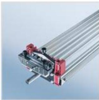
Sefar purchases the weaving accessories it needs for processing sensitive warp yarns from Groz-Beckert. For the highest weaving densities, 12-row warp stop motions are used. Carbon-fiber reinforced hybrid heald frames from Groz-Beckert enable Sefar to weave at widths of up to 430 cm without intermediate struts getting in the way. For
